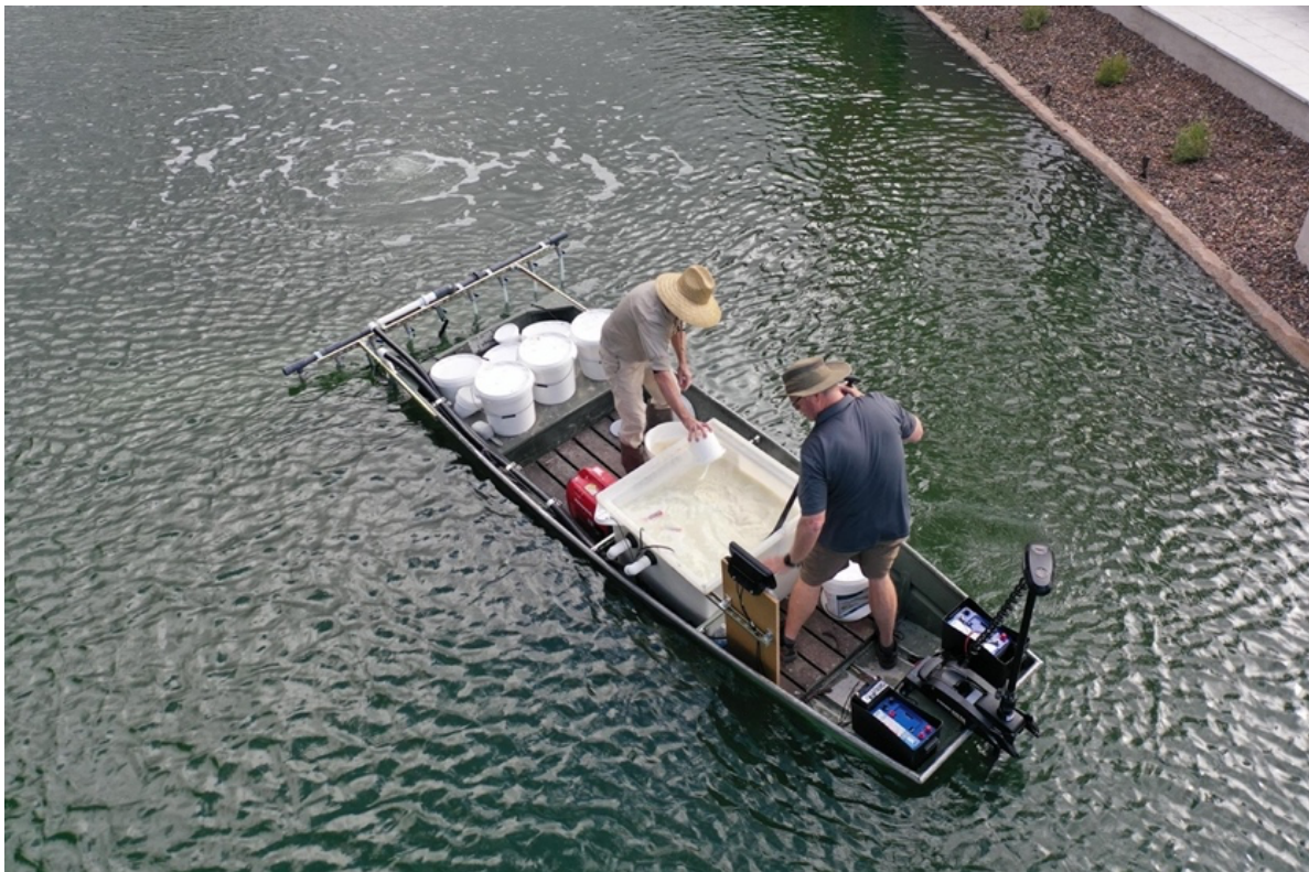
Boat with mixing chamber and product slurry ejection system
